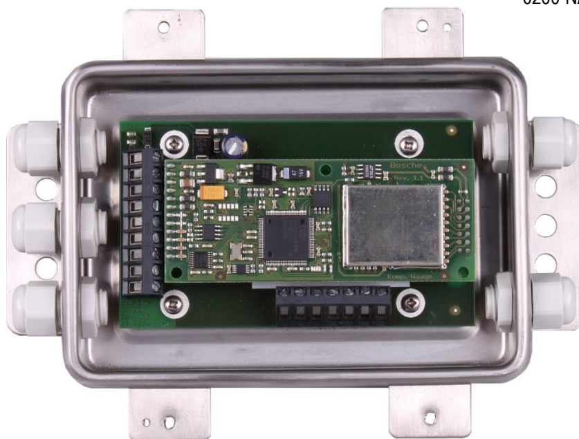
Figure 7a BDU10-M analog to digital data processing unit placed in a junction box as a weight transmitter.
