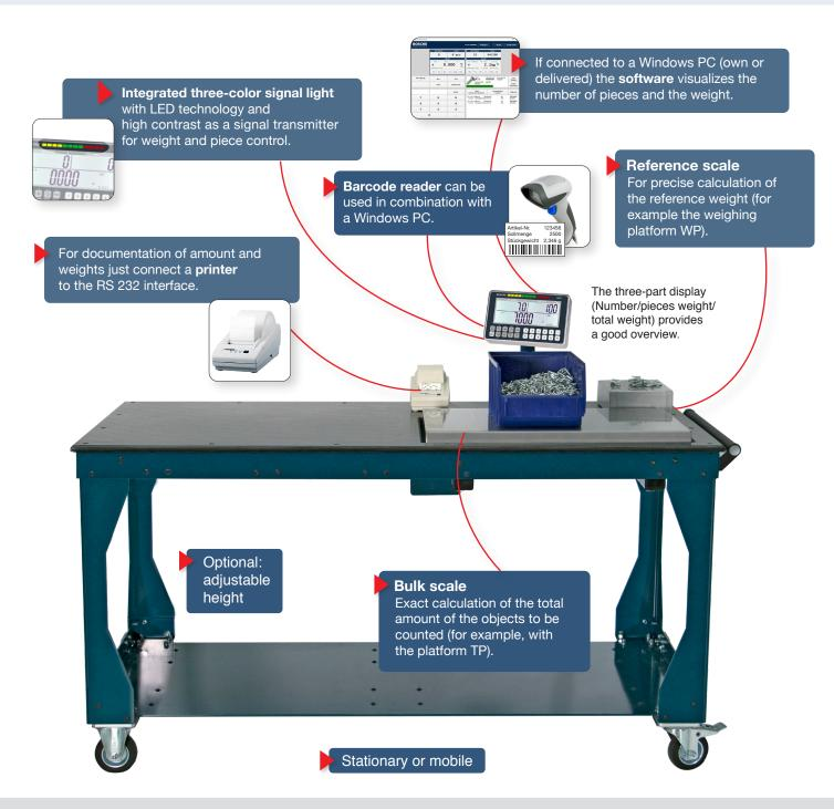
You can build your indivicual counting scale system by selecting different platforms from our range and combine these with our powerful counting indicator MCI for fast and precise counting. **Fast - Accurate - Noiseless.**
