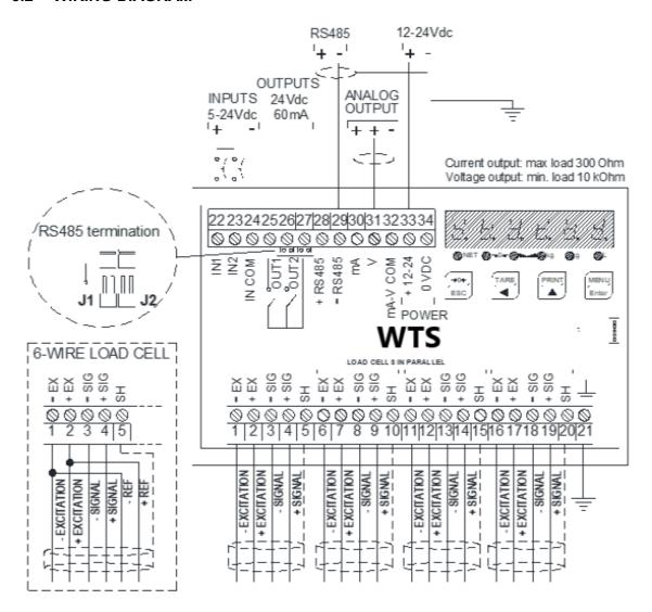
2 outputs: settable setpoints or remote output management via protocol.
